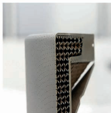
Several thousand slit and punctiform nozzles are printed into the cavity surface (left). Behind the mold wall there is the lattice structure (right), which also forms the space for the steam chamber and cooling water feed © Hofmann
